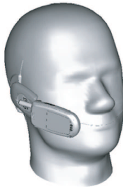
Figure 1. Complete model used for simulation including handset and SAM phantom head.
