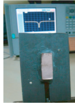
Figure 5. Photograph of fabricated proposed compact RDRA before attaching aluminum ground.
