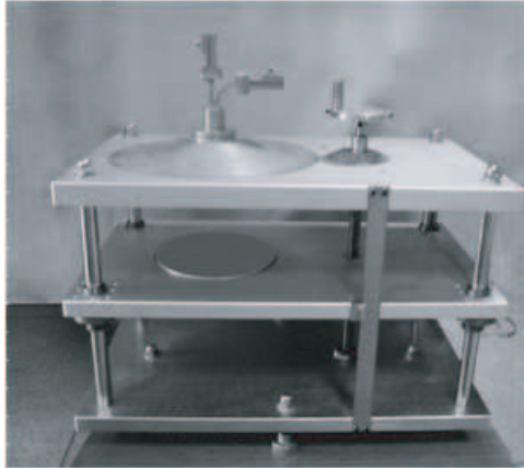
Figure 2. The configuration of the open resonator.
