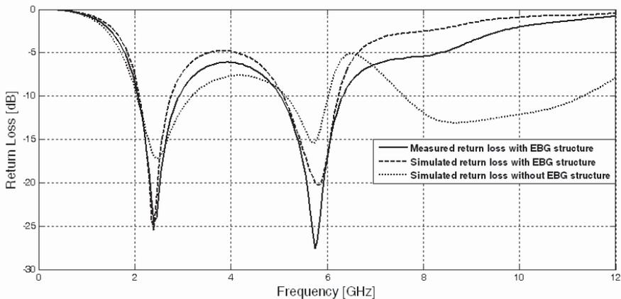
**Figure 3.** Simulated and measured return loss of the proposed antenna.
