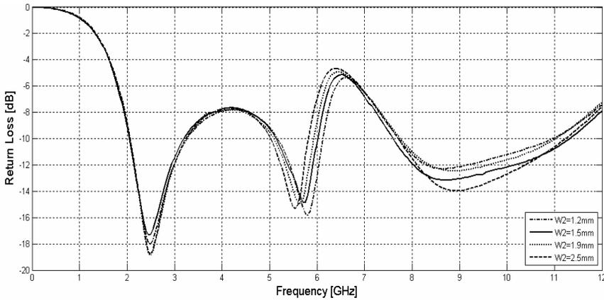
**Figure 6.** The effect on return loss due to the change of  $W_2$ .
