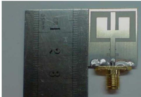
**Figure 2.** Photograph of the antenna.
