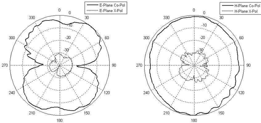
**Figure 9.** Measured radiation patterns of proposed antenna at 5.2 GHz.
