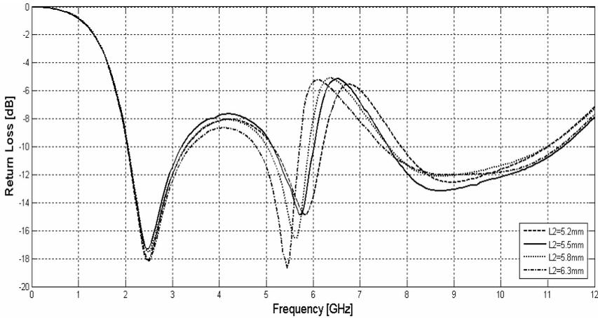
**Figure 4.** The effect on return loss due to the change of  $L_2$ .
