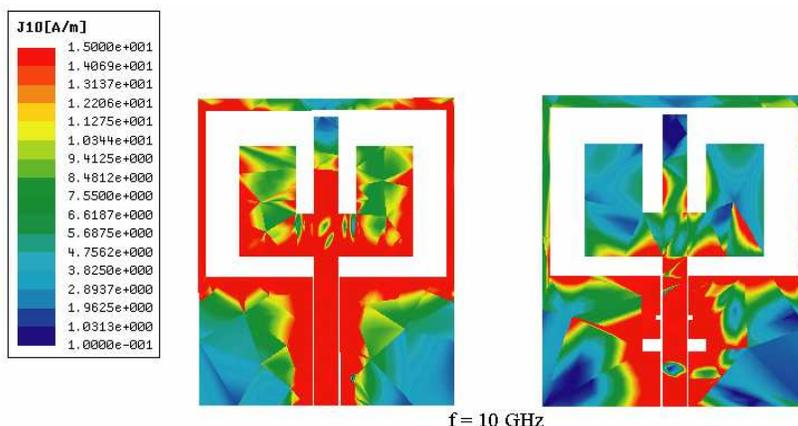
Figure 7. Electric current distribution over the substrate surface.
