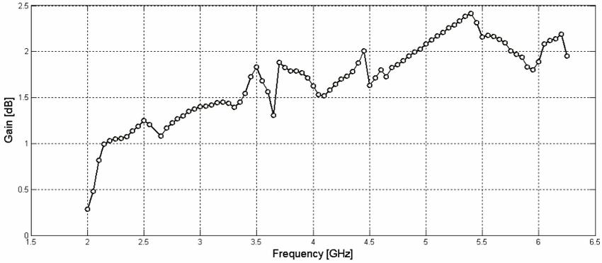
Figure 11. Simulated antenna gains for proposed antenna.
