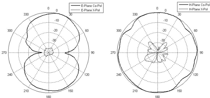
Figure 8. Measured radiation patterns of proposed antenna at 2.45 GHz.
