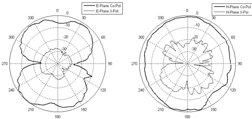
**Figure 10.** Measured radiation patterns of proposed antenna at 5.8 GHz.
