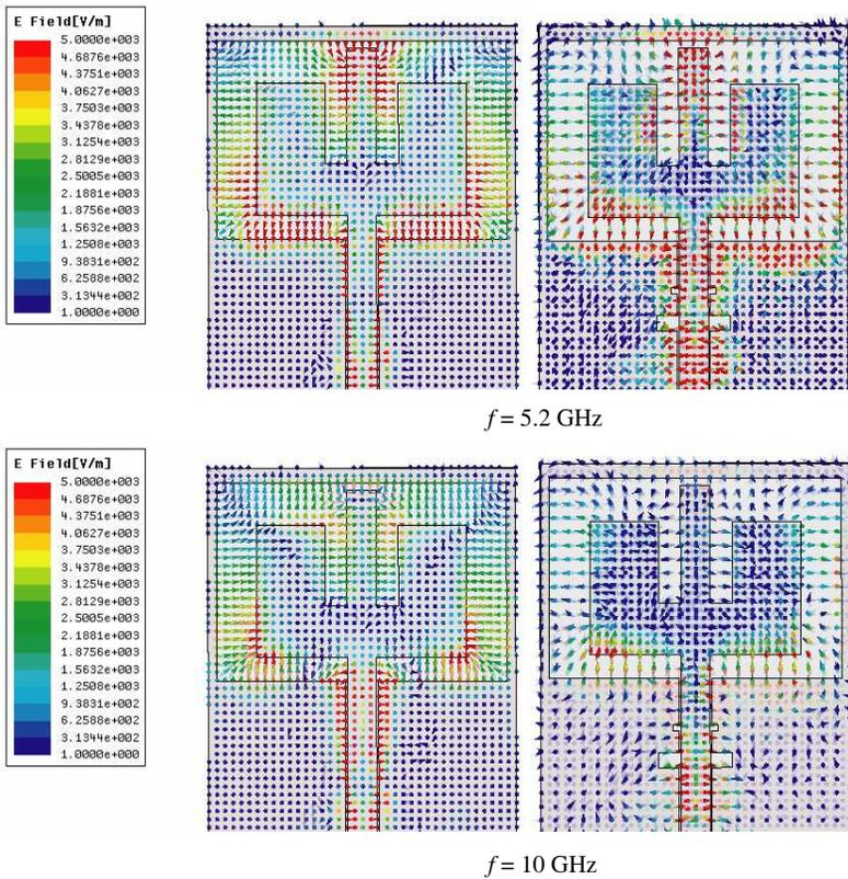
Figure 12. Electric field distribution of the antenna at 5.2 and 10 GHz.
