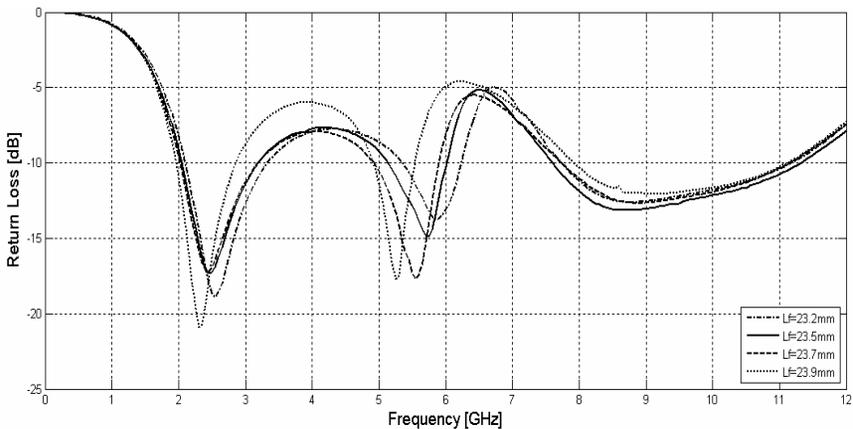
**Figure 5.** The effect on return loss due to the change of  $L_f$ .
