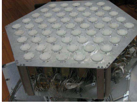
Figure 2. Photograph of SHA and RF front ends.
