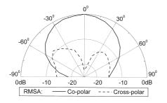
Figure 11. Radiation pattern of RMSA.
