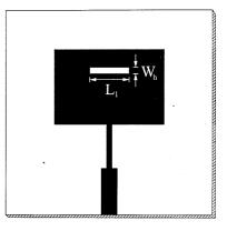
Figure 2. Geometry of WRMSA.
