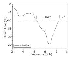
**Figure 9.** Variation of return loss versus frequency of CRMSA.
