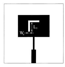
Figure 3. Geometry of ILRMSA.
