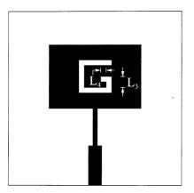
Figure 5. Geometry of GRMSA.
