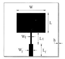
Figure 1. Geometry of RMSA.
