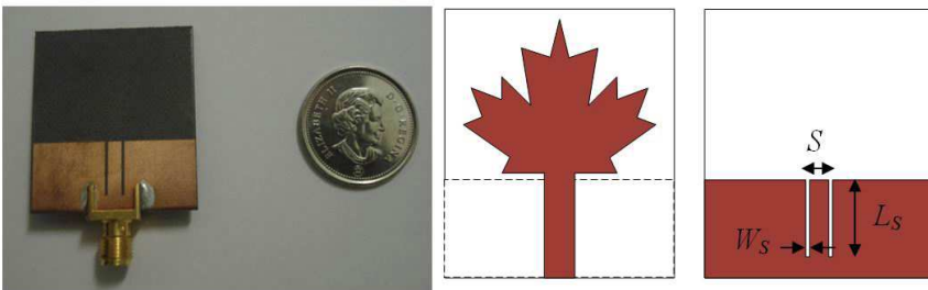
Figure 7. Geometry and photograph of the proposed bandstop antenna using two slits.
