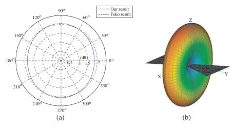
Figure 5. (a) A comparison between the resulting gain radiation pattern in x-z plane employing the MoM-based Feko technique and the results obtained via our program for optimized bow-tie antenna using BSO-NM (h = 21.078, d = 3.4818, and  $\alpha = 48.555^{\circ}$ ) at 2.45 GHz. (b) 3D Radiation pattern for an optimized bowtie antenna using BSO-NM (h = 21.078, d = 3.4818, and  $\alpha = 48.555^{\circ}$ ) at 2.45 GHz.
