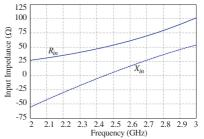
Figure 4. Input impedance versus frequency for an optimized bowtie antenna using BSO-NM (h = 21.078, d = 3.4818, and  $\alpha = 48.555^{\circ}$ ).
