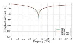
**Figure 3.** Reflection coefficient comparison for optimized bow-tie antenna using BFA, BSO, BFA-NM, BSO-NM algorithms.
