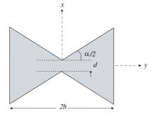
Figure 1. Geometry of bowtie antenna.
