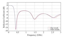
Figure 2. Reflection coefficient comparison between our result and Feko result for a bow-tie antenna  $(h = 10 \text{ cm}, d = 1 \text{ cm}, \text{ and } \alpha = 90^{\circ}).$
