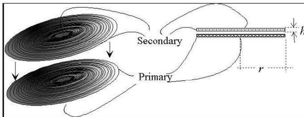
**Figure 1.** Air core planar transformer.
