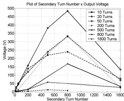
**Figure 5.** Graph showing peak resonance on transformers built with planar coils.
