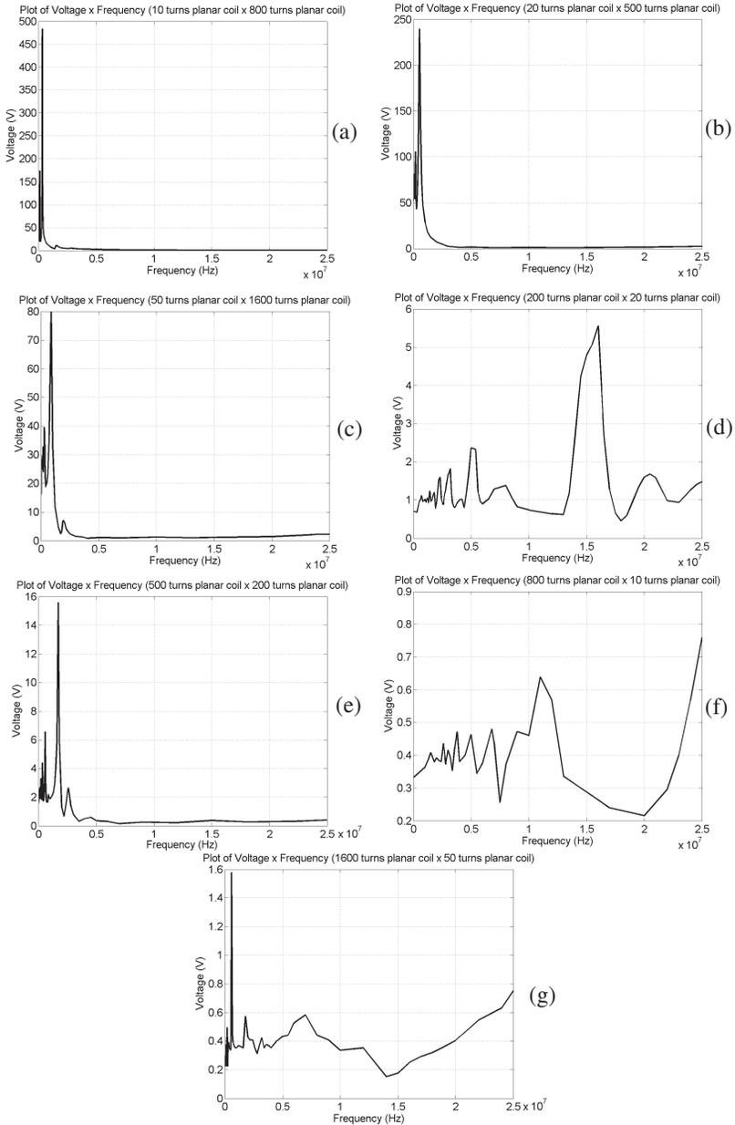
**Figure 4.** System Resonance for configurations: (a)  $10 \times 800$ ; (b)  $20 \times 500$ ; (c)  $50 \times 1600$ ; (d)  $200 \times 20$ ; (e)  $500 \times 200$ ; (f)  $800 \times 10$  and (g)  $1600 \times 50$ .
