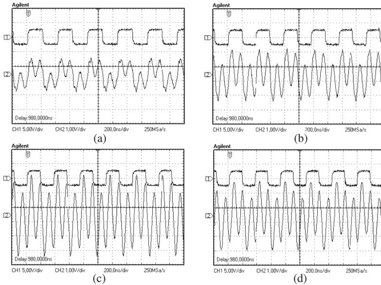
**Figure 3.** Planar  $\times$  planar transformer (configuration  $200 \times 50$ ) and sum of responses in phase in accordance to frequency of the square wave: (a)  $f = 2.4$  MHz; (b) 2.6 MHz; (c) 2.73 MHz ( $f_s = f_r/n$ ) and (d) 2.8 MHz.
