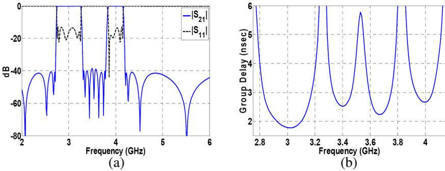
Figure 20. Dual-band filter design. (a) Frequency and (b) group delay response.
