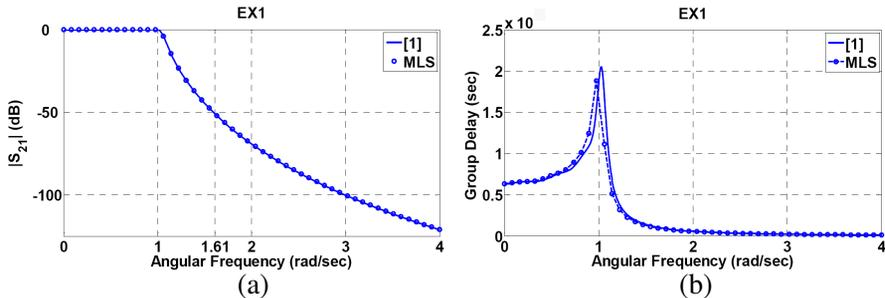
Figure 6. Example 1. (a) Transmission and (b) group delay versus angular frequency.
