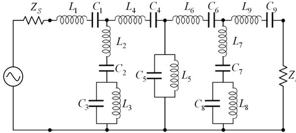
**Figure 15.** Circuit diagram of the BP filter in example 6.
