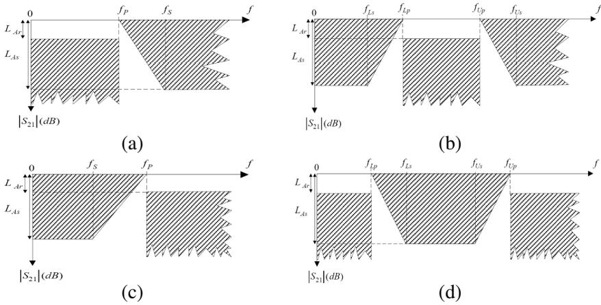
**Figure 2.** Diagrams of design specifications: (a) Lowpass, (b) bandpass, (c) highpass and (d) bandstop.
