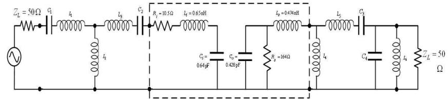
Figure 21. Prototype of input and output highpass filter for matching in pass band.
