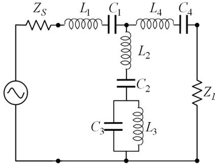
Figure 13. Circuit diagram of the BP Filter in Example 5.
