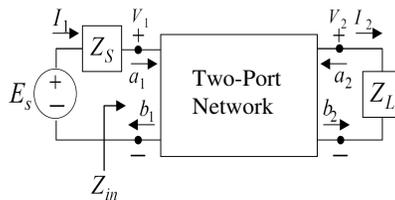
**Figure 1.** Schematic diagram of a two port network.
