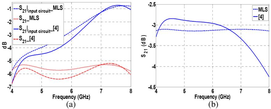
**Figure 22.** Design of impedance matching circuits of a transistor equivalent circuit. (a) Input BP filter response, (b) output BP filter response.
