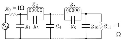
Figure 9. Circuit configuration of example 3.
