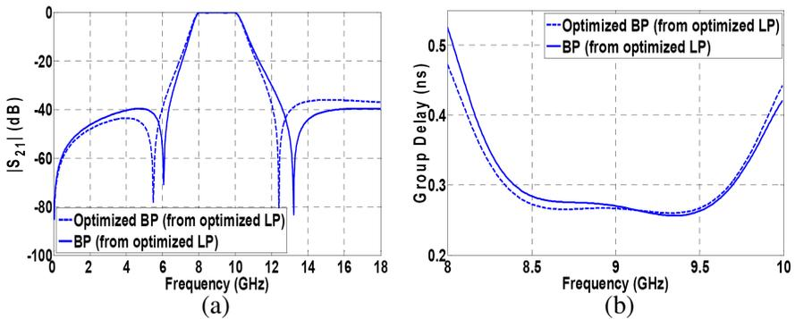
Figure 14. Comparison of performance of BP filter as derived from the optimized LP filter and further optimization of BP filter from optimized lowpass case to bandpass; (a)  $|S_{21}|$  dB. (b) Group delay.
