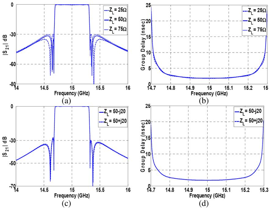
**Figure 16.** Example 6. (a) Frequency and (b) group delay response of bandpass filters with real load impedances. (c) Frequency and (d) group delay response of BP filters with complex load impedances.
