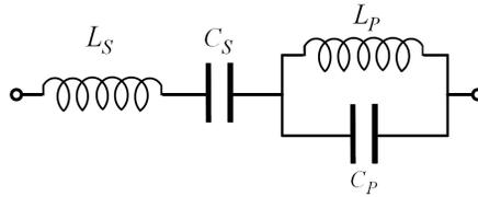
**Figure 3.** The schematic diagram of a circuit unit in a branch.
