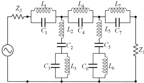
**Figure 17.** Prototype for band stop design.
