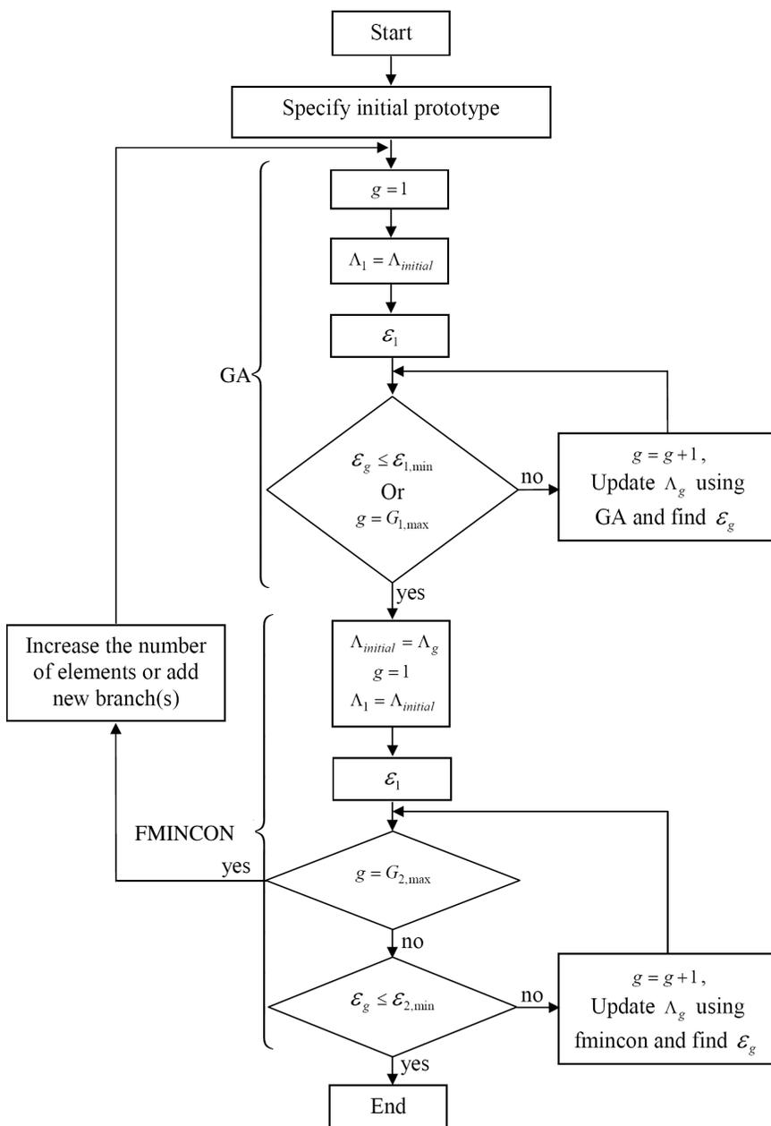
**Figure 4.** Flowchart of the MLS algorithm for the optimization of filter element values.
