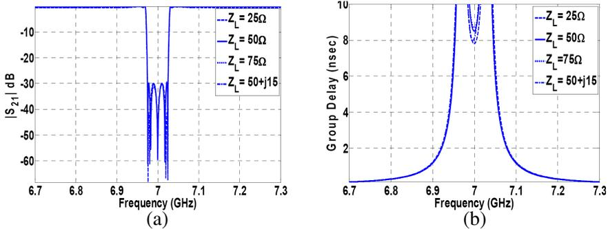
**Figure 18.** BS filter design for (a) different load impedances and related (b) group delays of the circuit in Fig. 17.
