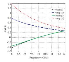
Figure 5. The real and imaginary parts of  $\varepsilon$ ,  $\mu$  versus frequency.
