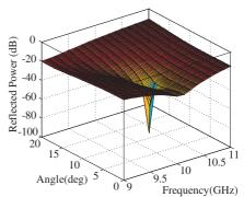
Figure 2. Reflected power (in dB) from the structure in Fig. 1(a) with characteristic given in example 1 versus the angle of incidence at frequencies f=12, 10,  $20\,\text{GHz}$  for TE polarization.
