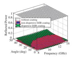
**Figure 8.** 3-D diagram of reflected power from a PEC plane versus frequency and angle of incidence under oblique incidence of a TM plane wave for three cases: (a) without coating. (b) With two layers of nondispersive DZR metamaterial coatings with characteristics given in Eq. (28). (c) With two layers of dispersive DZR metamaterial coatings with characteristics given in Eq. (29).
