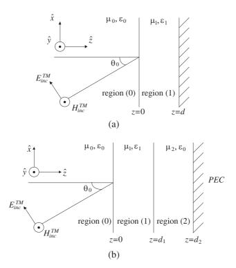
**Figure 1.** A perfect electric conducting (PEC) plate covered by DZR metamaterial layers.
