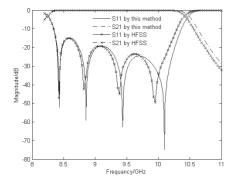
Figure 10. Magnitude compared with CAD software HFSS.
