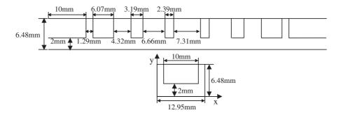
Figure 7. Rectangular single-ridged waveguide filter.
