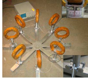
Figure 7. Schematic diagram of the manufactured MTC composed of 8 SCS.
