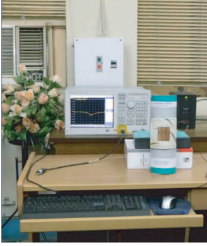
Figure 14. Snapshot of S_{11} measurement set up.
