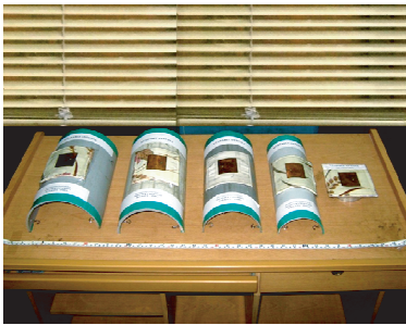
Figure 13. Photograph of the various antenna structures bent with different radii.
