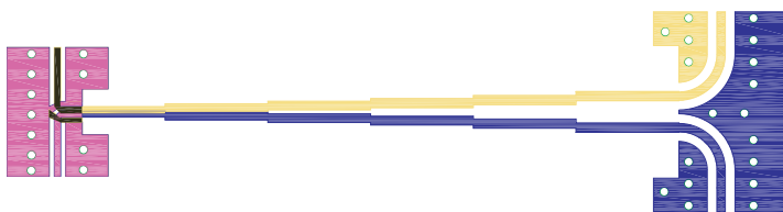
Figure 8. Top view of directional couplers with the novel mixed first section and SMCPW bends.
