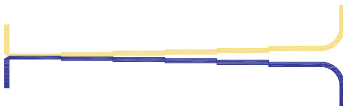
Figure 3. Top view of directional couplers with access stripline ports. Swept bends and 90° mitered bends are used at the weakly and tightly coupled sections, respectively.
