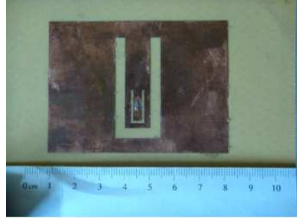
Figure 10. Photograph of the fabricated antenna with two U-slots.
