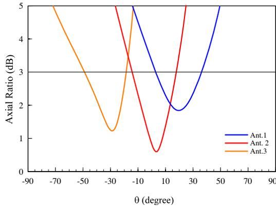
**Figure 6.** AR against  $\theta$  degree in  $y$ - $z$  plane of the proposed CP antenna at  $f_c$ .
