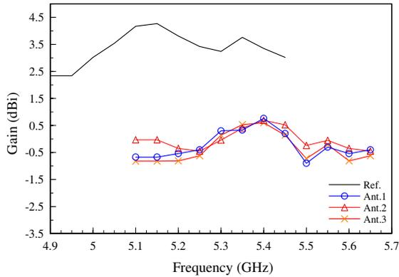
**Figure 8.** Measured antenna gain for Ref., Ant. 1, Ant. 2, and Ant. 3 in frequency.
