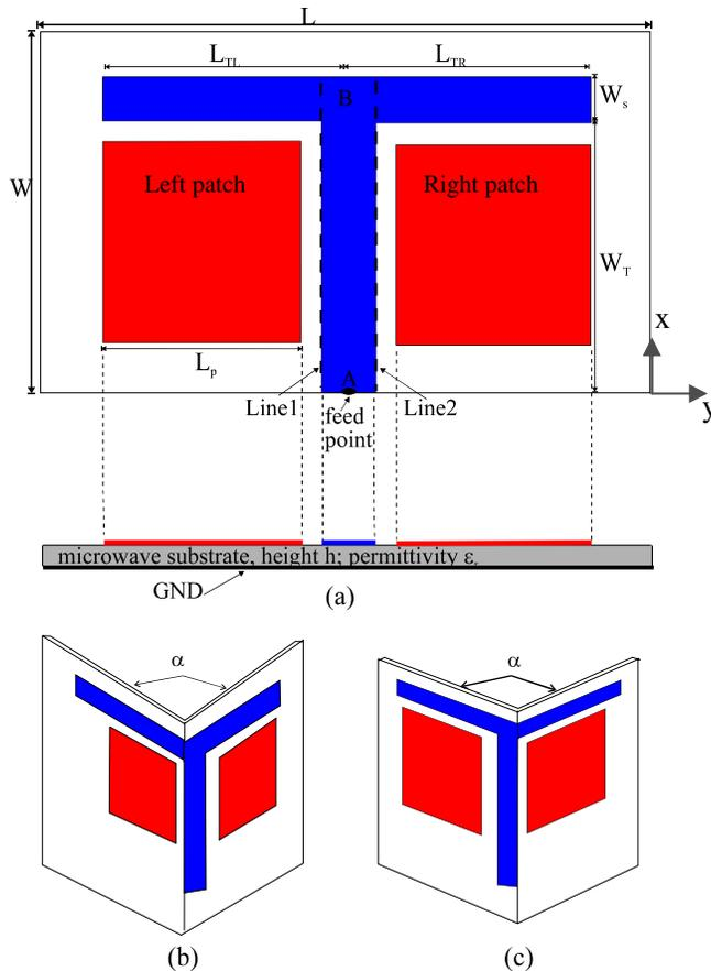
**Figure 1.** Configuration of the proposed antenna in sense of (a) linear polarization, (b) right-handed circular polarization, and (c) left-handed circular polarization.
