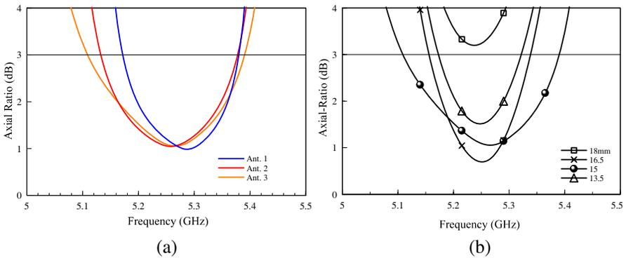
**Figure 7.** Simulated Axial Ratio in frequency with varied (a)  $\alpha$ , and (b)  $L_{LT}$ .
