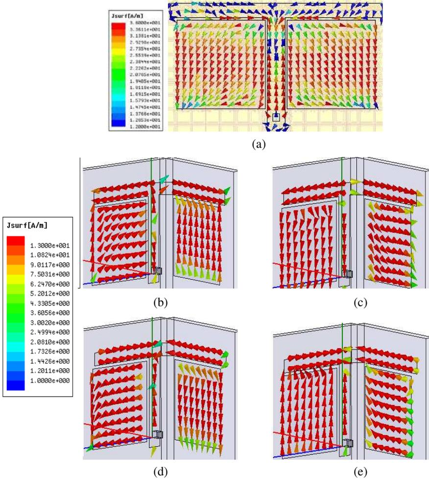
**Figure 4.** (a) Simulated surface currents on patches and T-strip at 5.2 GHz for Ref.. Simulated surface currents on patches and T-strip at 5.2 GHz for Ant. 3 in phase of (b) 0°, (c) 90°, (d) 180°, and (e) 270°.
