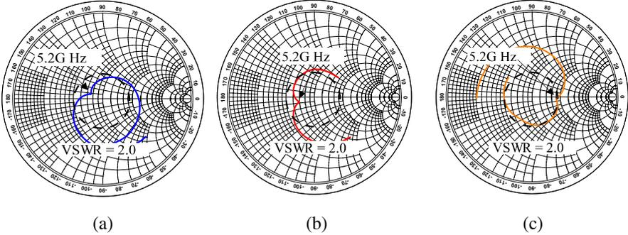
**Figure 3.** Measured Smith chart at center operating frequency for (a) Ant. 1, (b) Ant. 2, and (c) Ant. 3.
