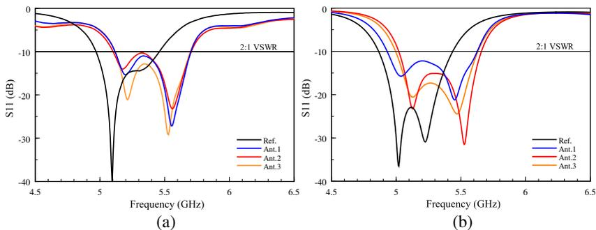
**Figure 2.**  $S_{11}$  in frequency of four studied prototypes. (a) Measurement; (b) Simulation. The simulations performed with the commercial microwave software of Ansoft HFSS 10.0.
