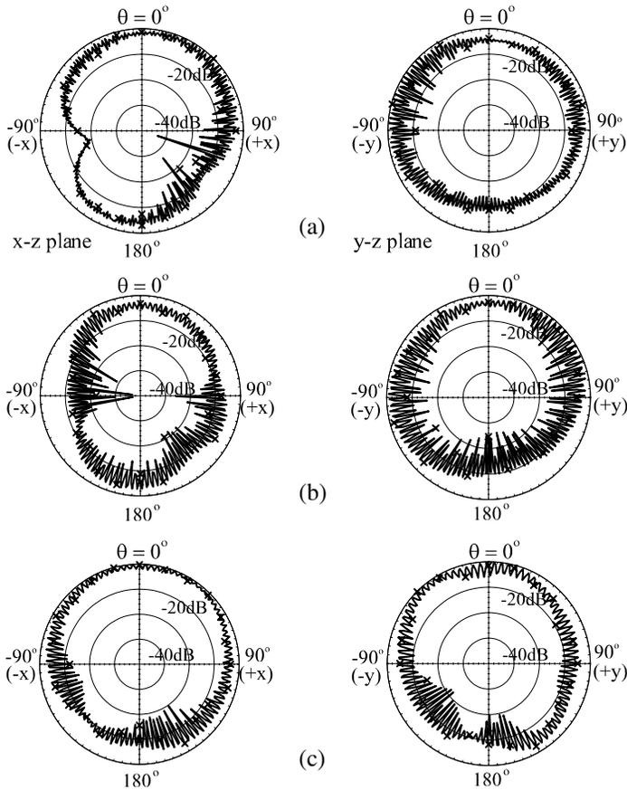
**Figure 5.** Measured linear spinning patterns at  $f_c$  for (a) Ant. 1, (b) Ant. 2, and (c) Ant. 3.
