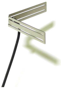
Figure 2. Photo of a constructed prototype made of a 0.3\text{-mm} thick alloy and fed by a 50\text{-}\Omega mini-coaxial cable.
