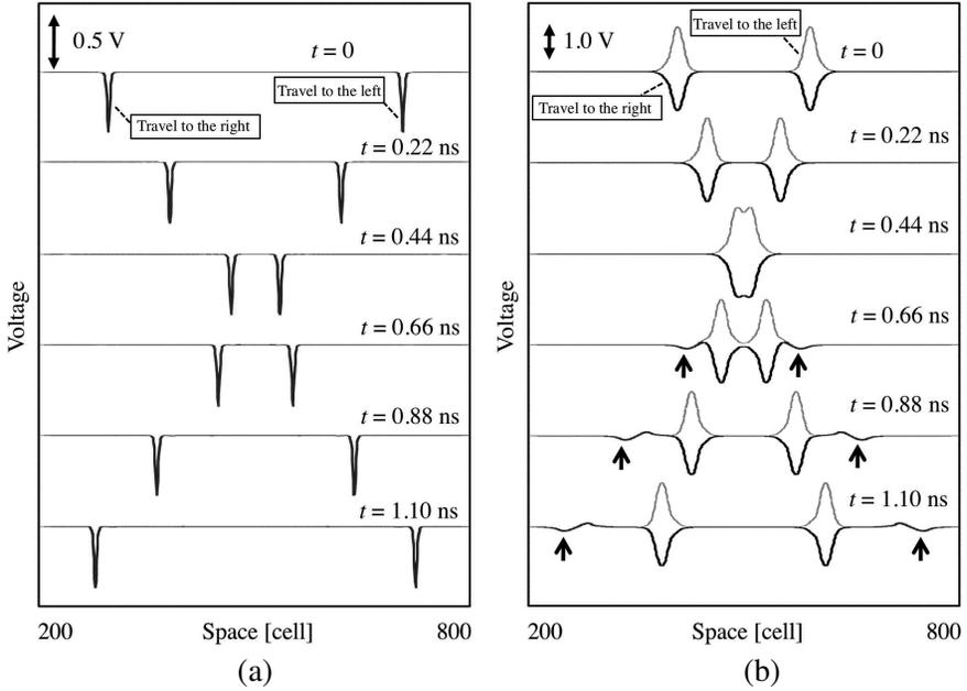
**Figure 2.** Interaction of two nonlinear pulses on a coupled NLTL. (a) The colliding  $c$ -mode nonlinear pulses and (b) the colliding  $\pi$ -mode nonlinear pulses. The arrows in Fig. 2(b) indicate the  $c$ -mode pulses generated by colliding two  $\pi$ -mode pulses traveling in the opposite directions.
