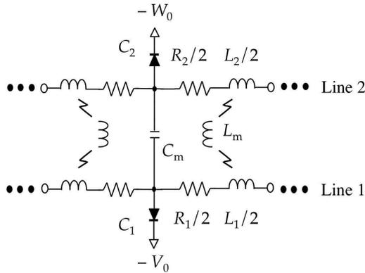
**Figure 1.** The unit cell of a coupled NLTL.
