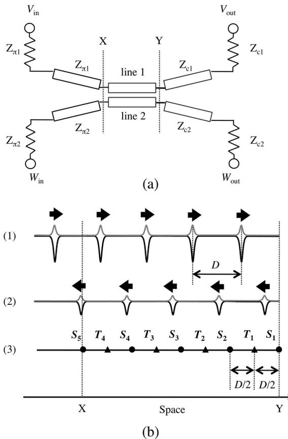
**Figure 3.** The method for increasing the repetition rate of incident pulse stream using coupled NLTLs. (a) The circuit configuration and (b) the operating principle.
