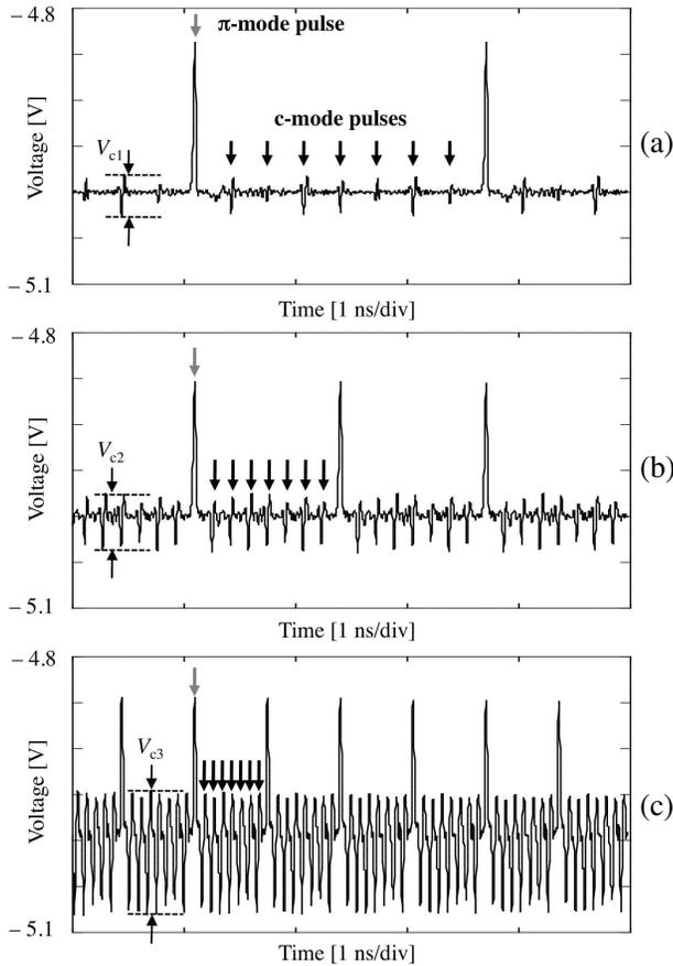
**Figure 4.** Numerical demonstration of increasing the repetition rate of incident pulse stream. The output waveforms at the repetition-period of (a) 2.616, (b) 1.308 and (c) 0.654 ns. Grey and black arrows indicate the incident  $\pi$ -mode pulses and newly developing  $c$ -mode pulses, respectively.
