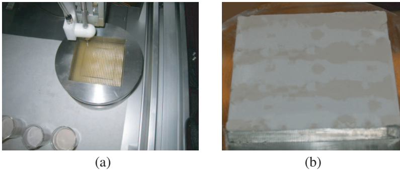
Figure 17. (a) Automated dispensing machine for DPD in action when depositing available ceramic powder constituents into desired material distribution for the 3 \times 3 array of the unit cell discretized into 9 \times 9 design variable configuration shown in Figure 16(a) resulting in (b) a desired deposited substrate.
