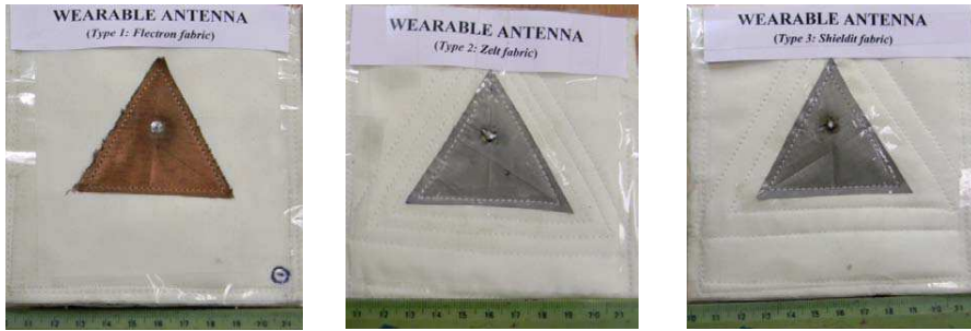
Figure 2. Photographs of electro-textile based WiBro antennas developed.
