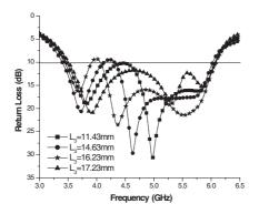
Figure 5. Effect of variation of slot length  $L_3$  on return loss.
