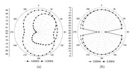
Figure 10. Radiation pattern plot of proposed antenna. (a) Azimuthal plane, (b) elevation plane.
