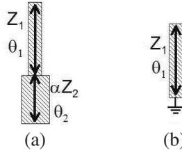
Figure 2. (a) Even mode resonator. (b) Odd mode resonator.
