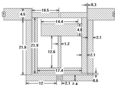
**Figure 7.** Dimensions in millimetres of fabricated second order filter.
