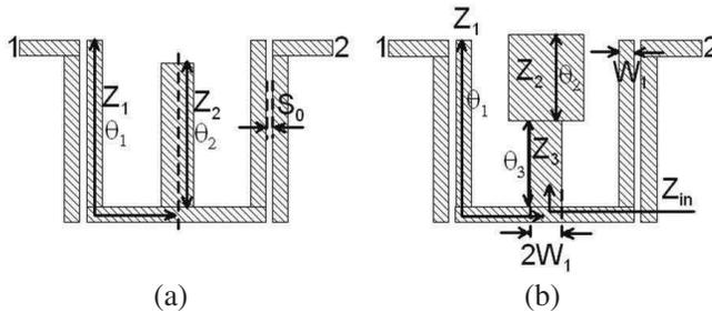
**Figure 1.** (a) Dual-mode resonator. (b) Stepped-impedance resonator.
