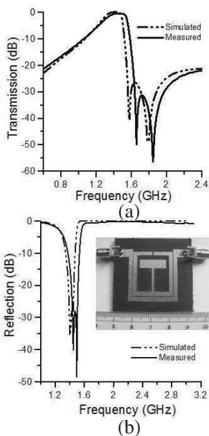
**Figure 8.** Simulated and measured  $S$ -parameters of fabricated filter.
