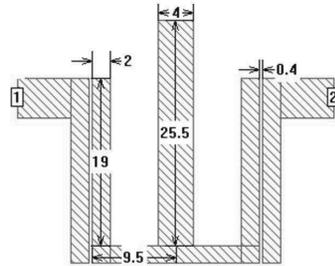
Figure 4. Layout and dimensions of designed filter in millimetres.
