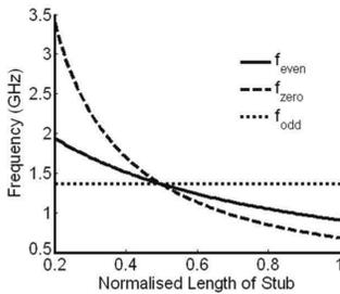
**Figure 5.** Variation of TZ and even mode pole with stub length.
