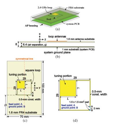
**Figure 1.** (a) Perspective drawing of the proposed printed loop antenna integrated into a compact outdoor AP. (b) Sectional view of the proposed design backed by a system PCB of an AP. (c) Geometry of the proposed loop antenna formed on a low-cost FR4 substrate. (d) Detailed dimensions of the loop antenna.
