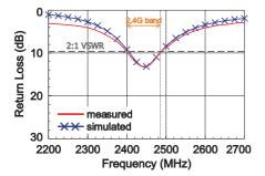
Figure 3. Measured and simulated return loss; D = 35.5 mm, L = 15 mm.
