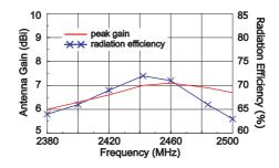
Figure 8. Measured peak antenna gain and radiation efficiency.
