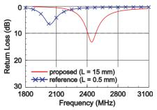
Figure 4. Simulated return loss for the proposed antenna with (L = 15 mm) and without (L = 0.5 mm) the tuning portion.
