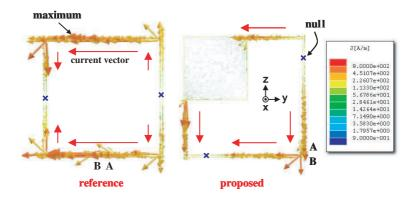
Figure 9. Simulated excited surface currents in the form of vectors at 2442 MHz on the proposed and the reference antennas.
