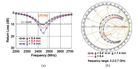
Figure 5. Simulated (a) return loss and (b) input impedance on the Smith chart as a function of the distance g of the air separation.
