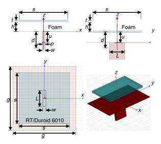
Figure 1. Antenna geometry and parameters.
