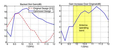
Figure 5. Computed gain using HFSS of the final design compared to the initial one.
