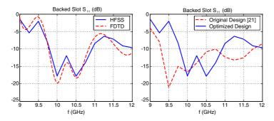
Figure 6. Return Loss for the final design compared to the initial one.
