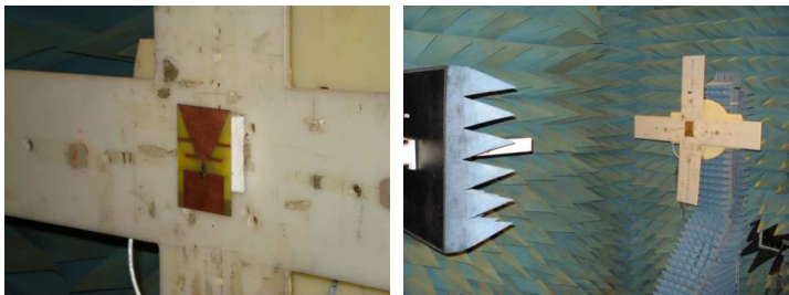
Figure 6. Measurement of proposed multi-band antenna's radiation pattern.
