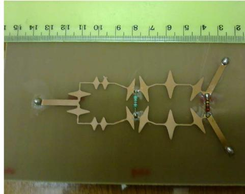
**Figure 8.** A photograph of the fabricated dual-frequency NTL-WPD.
