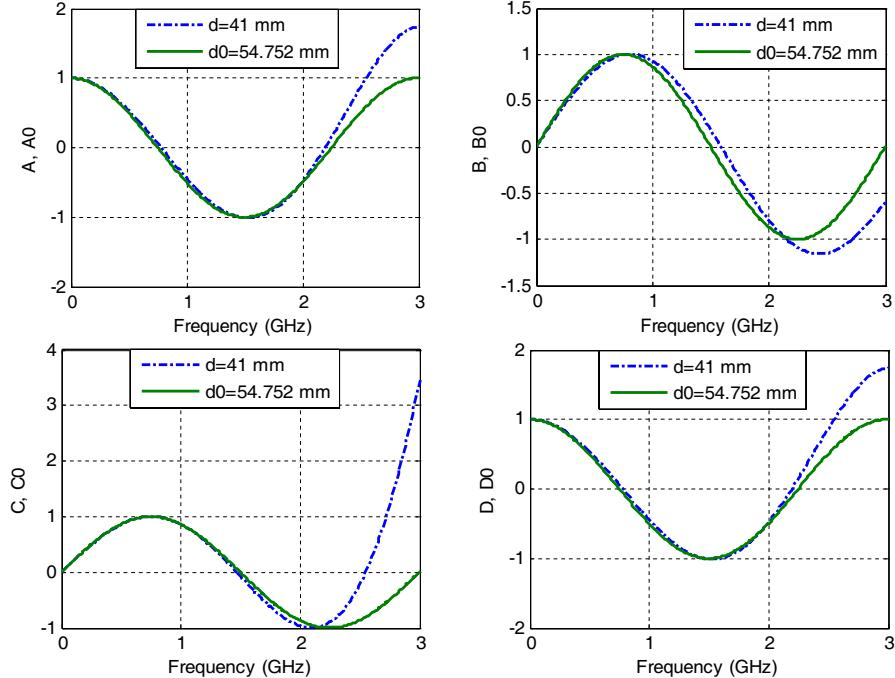
**Figure 4.** The ABCD parameters of  $Z_2(z)$  with an error of 0.075.
