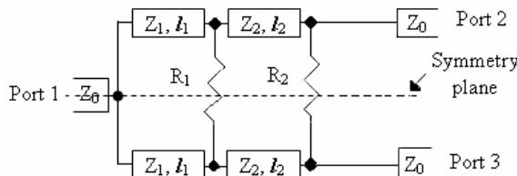
**Figure 2.** Dual-frequency WPD with two resistors [13].
