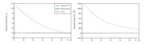
Figure 4. Percent errors of the skin effect internal impedance ratios of approximate formulas relative to the truncated exact formula for tubular cylindrical conductors with a radius ratio s = 0.95.
