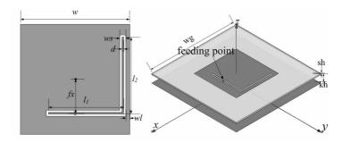
Figure 6. Broadband microstrip antennas with L-shaped coplanar feed-line.
