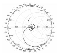
**Figure 7.** Measured and simulated reflection coefficient for the antennas with L-shaped coplanar feed-line.
