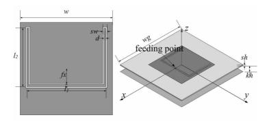
Figure 1. Broadband microstrip antennas with U-shaped coplanar feed-line.
