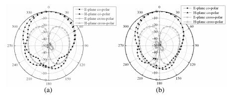
Figure 4. Measured radiation patterns for the antennas with U-shaped coplanar feed-line.
