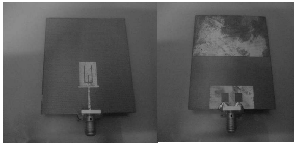
Figure 4. Front and back views of the UWB antenna with band-notch.
