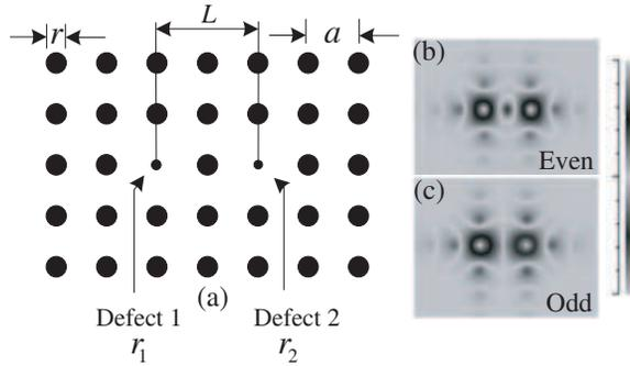
**Figure 2.** (a) Structure of two coupled resonators formed by point defects. And electric field profiles of two states of two coupled resonators: (b) even mode, (c) odd mode.
