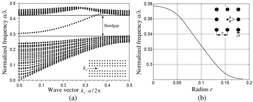
**Figure 4.** (a) Dispersion diagram of the guided mode inside the PBG (photonic band gap) in the  $\Gamma$ - $X$  direction. (b) Dependence of the resonant frequency of the coupled cavity on the coupled defect radii.
