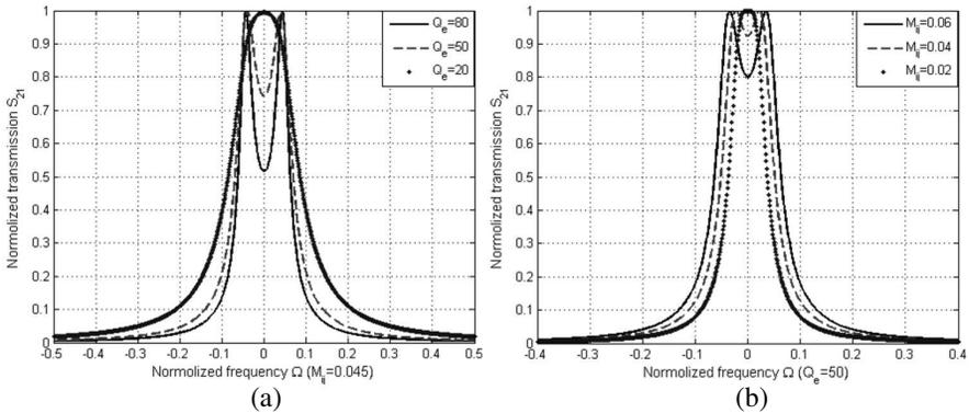
**Figure 3.** Comparison of the transmission spectra of the coupled cavities filter with different parameters. (a) Different external quality factors:  $Q_e = 20$  (dot line),  $Q_e = 50$  (dash line), and  $Q_e = 80$  (solid line). (b) Different coupling coefficients:  $M_{ij} = 0.02$  (dot line),  $M_{ij} = 0.04$  (dash line),  $M_{ij} = 0.06$  (solid line).
