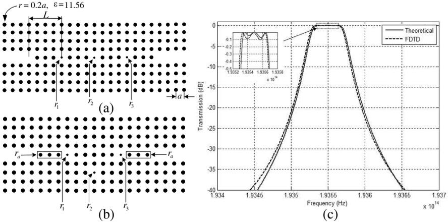
**Figure 5.** (a), (b) Schematic diagram of the designed filter, which is composed of 3 resonators. (c) Transmission spectra of the desired filter by the synthesized method (real line) and the simulation result by the FDTD method (dotted line).
