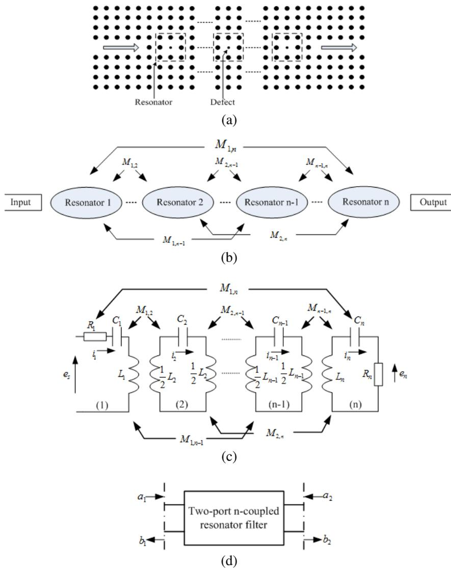
**Figure 1.** (a) Structure of the coupled resonator filter in a PC, which is composed of  $n$  resonators. (b) Schematic diagram of the filter. (c) Equivalent circuit of the structure in (a). (d) Its network representation.
