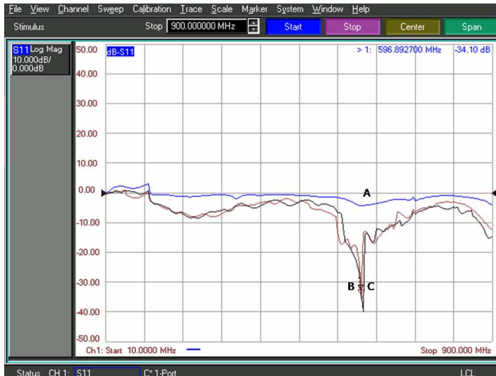
Figure 7. Response at 200 Hz AC voltage shows efficient antenna characteristics with sharply defined resonant frequency.
