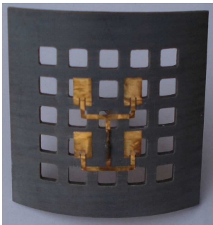
Figure 10. Fabricated cylindrical conformal array antenna with PBG lattice.
