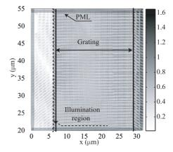
Figure 3. Time step picture of a diffraction grating simulation.
