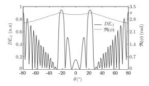
Figure 2. Real part of  $\phi$  and the reflectance as a function of the angle of incidence. The parameters of the grating where:  $\Lambda = 0.2 \,\mu\text{m}$ ,  $d = 15 \,\mu\text{m}$ ,  $\Delta n = 0.025$  and  $\lambda = 633 \,\text{nm}$ .
