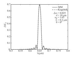
Figure 5. Diffraction efficiency as a function of the wavelength for grating with the following parameters:  $\Lambda = 0.2 \,\mu\text{m}, d =$  $10 \,\mu\text{m}, n_0 = 1.63, \,\Delta n = 0.025, \,\theta = 0^{\circ}.$
