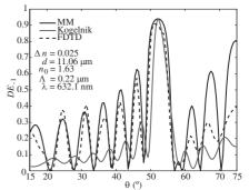
Figure 6. Diffraction efficiency as a function of the angle of incidence. Comparision between Mathieu's theory, Kogelnik's theory and also the FDTD method.
