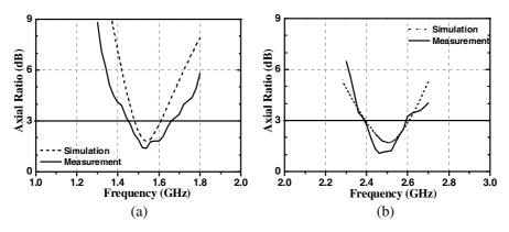
Figure 4. Axial ratio spectrums (a) 1.57 GHz, (b) 2.46 GHz.
