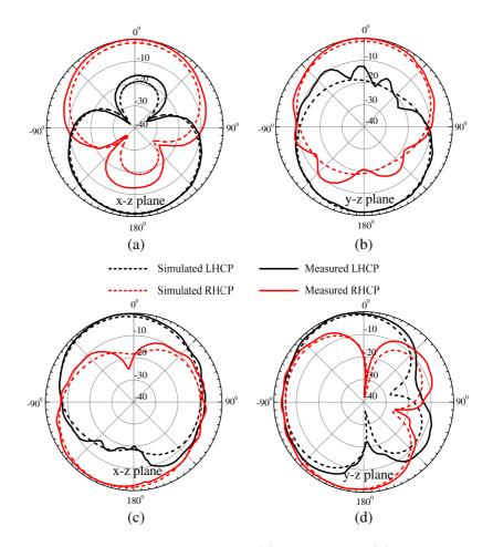
Figure 7. Radiation patterns: (a) x-z plane, (b) y-z plane at 1.57 GHz, (c) x-z plane, (d) y-z plane at 2.46 GHz.
