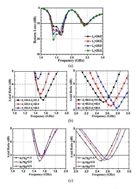
**Figure 2.** Characteristics of the parameter variations. (a) Variation of feed strip length. (b) Variation of radius of two opened-ground rings. (c) Variation of gaps of two opened-ground rings.
