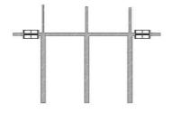
Figure 5. Layout of Rx-filter with SCMRC.
