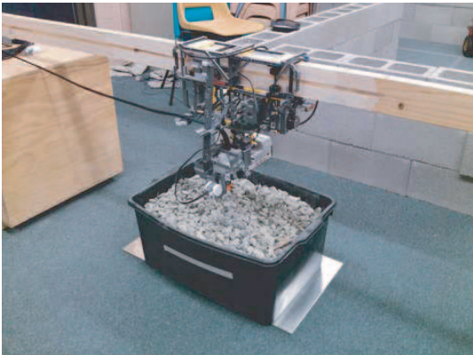
Figure 6. Experimental setup to capture VOF data over rock samples.
