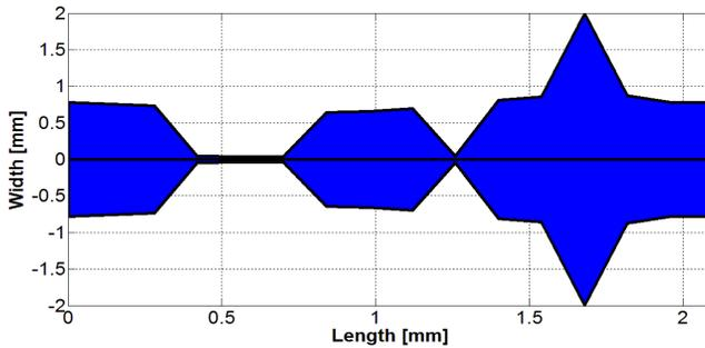
**Figure 10.** Example of a filter profile with the microstrip of  $150\ \Omega$  (0.08 mm).
