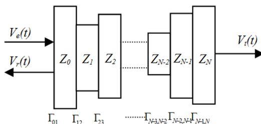
Figure 4. Example of a transmission line filter.
