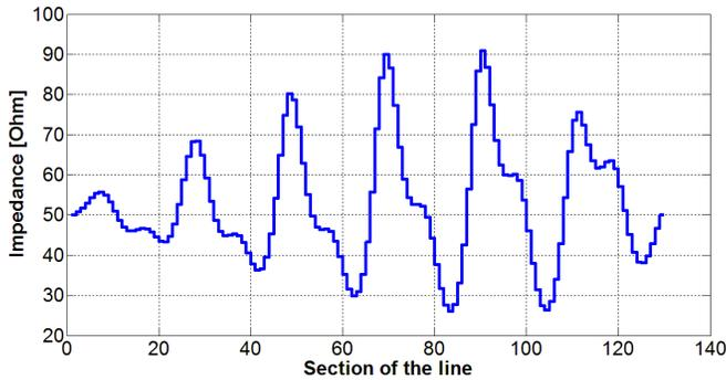
**Figure 5.** Impedance profile of the filter.
