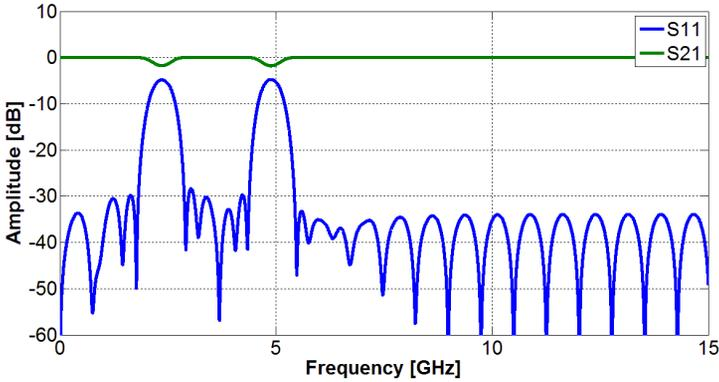
**Figure 9.** The  $S$  parameters without compensation.
