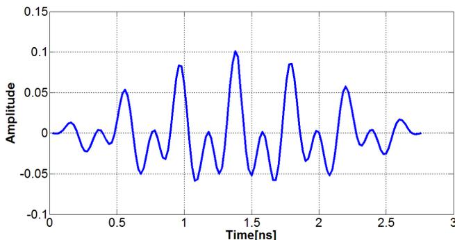
Figure 3. Reflected wave of the ideal filter.
