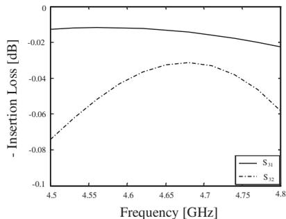
**Figure 4.** Insertion loss with respect to frequency of the STCWB-OMT for vertical and horizontal polarizations.
