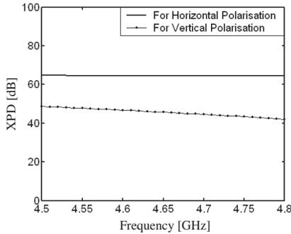
**Figure 5.** Cross-polarisation discrimination (XPD) with respect to frequency of the STCWB-OMT for vertical and horizontal polarizations.
