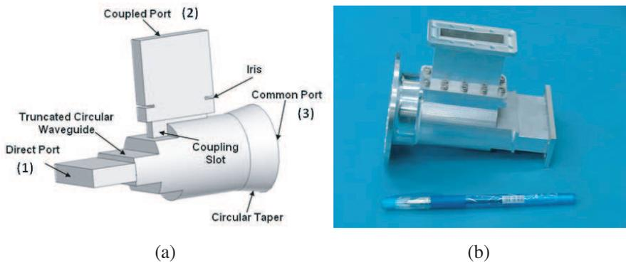
**Figure 1.** Stepped Truncated-Circular Waveguide Branching Ortho-Mode Transducer (STCWB-OMT). (a) Synthesized geometry. (b) Photograph.
