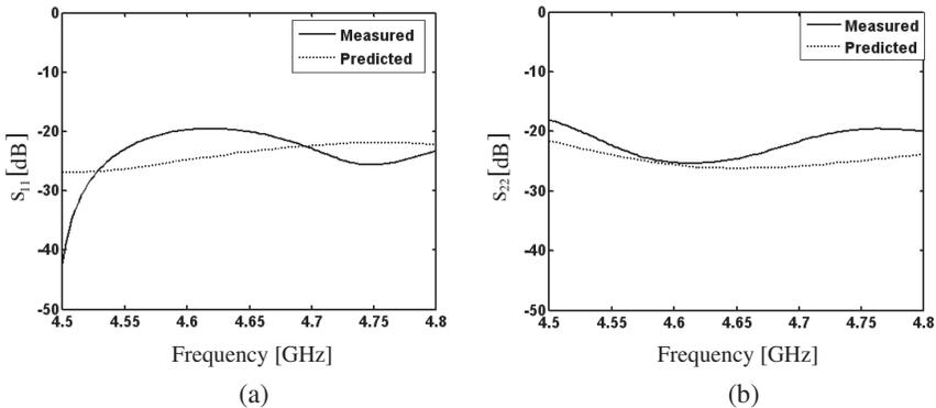
**Figure 2.** Predicted and measured return loss versus frequency of the STCWB-OMT at (a) direct port and (b) coupled port.
