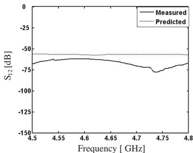
**Figure 3.** Predicted and measured port-port isolation versus frequency of the STCWB-OMT.
