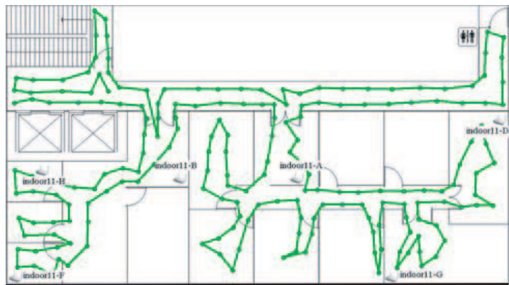
Figure 9. The survey trail and AP placement of experimental testbed.
