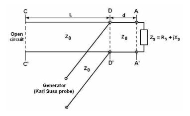
Figure 4. Equivalent geometry of the probe-tip position in Figure 3.
