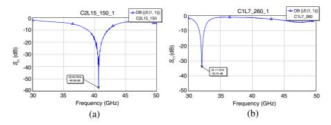
Figure 5. Return loss measurement of the of CRLH antenna radiating structures made (a) on silicon and (b) on alumina substrate.
