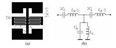
Figure 1. Layout of the CPW CRLH elementary cell used in (a) antenna construction and (b) its equivalent circuit.
