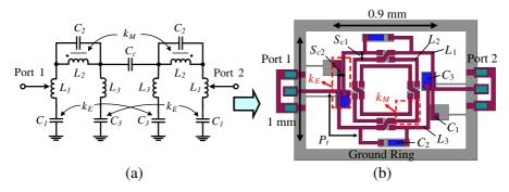
**Figure 12.** Proposed transformer-coupled dual-band bandpass filter design using glass IPD technology. (a) Equivalent circuit. (b) Corresponding layout structure.
