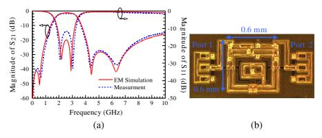
Figure 9. Results and structure of the designed IPD dual-mode bandpass filter. (a) Comparison of the magnitude of  $S_{21}$  and  $S_{11}$  between EM simulation and measurement. (b) Chip photograph.
