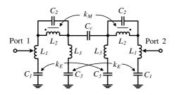
Figure 10. Equivalent circuit of the designed dual-band bandpass filter.
