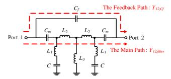
Figure 6. Equivalent circuit of dual-mode bandpass filter with a capacitive feedback path.
