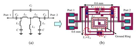
**Figure 8.** Proposed dual-mode bandpass filter design using glass IPD technology. (a) Equivalent circuit. (b) Corresponding layout structure.
