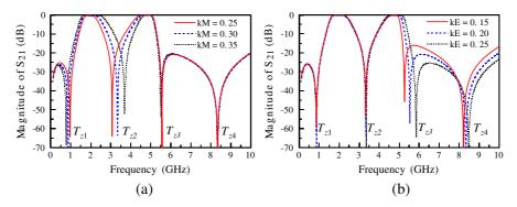
Figure 11. Comparison of the magnitude of  $S_{21}$  for the dual-band bandpass filter design with different electrical and magnetic coupling coefficients. (a) Magnitude of  $S_{21}$  with varying  $k_M$ . (b) Magnitude of  $S_{21}$  with varying  $k_E$ .
