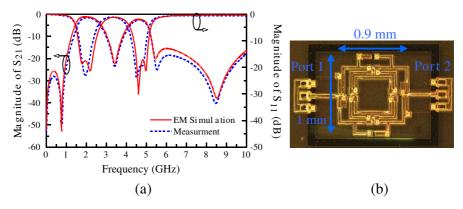
Figure 13. Results and structure of the designed IPD transformercoupled dual-band bandpass filter. (a) Comparison of the magnitude of  $S_{21}$  and  $S_{11}$  between EM simulation and measurement. (b) Chip photograph.
