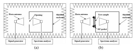
Figure 2. Experimental test setup used to determine shielding effectiveness. (a) Reference measurement (without sample) and (b) load measurement (with sample).
