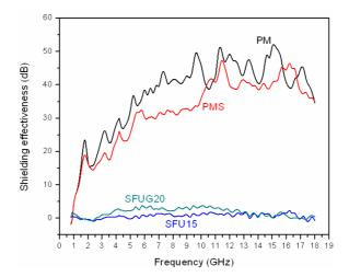
Figure 3. Shielding effectiveness in the 1–18 GHz range.
