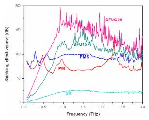
Figure 5. Shielding effectiveness in terahertz domain.
