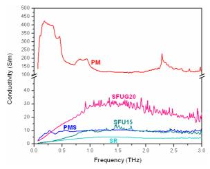
Figure 6. Samples conductivity in terahertz domain.
