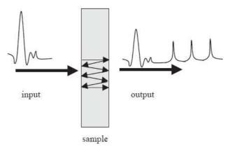
Figure 1. THz TDS spectroscopy.
