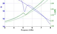
Figure 9. TX VCO inductor performance with and without aperture coupling.
