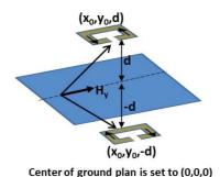
Figure 2. Image theory for case 1 (with no slot).
