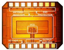
Figure 5. TX VCO chip microphotograph.
