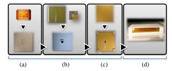
**Figure 10.** TX aperture coupled SoP (a) TX chip placed in LTCC substrate, (b) ground plane with slot and LTCC post placed on substrate with the TX chip, (c) superstrate with patch antenna placed on the rest of the module, (d) complete SoP module.
