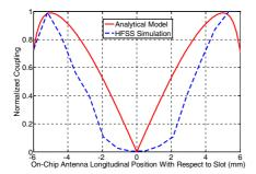
Figure 4. Comparison of coupling between the loop and the slot through HFSS and analytical model.
