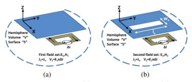
**Figure 1.** Problem definition (a) Case 1 with no slot, (b) Case 2 with slot.
