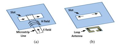
Figure 3. Comparison of coupling between a microstrip feed and a loop antenna feed.
