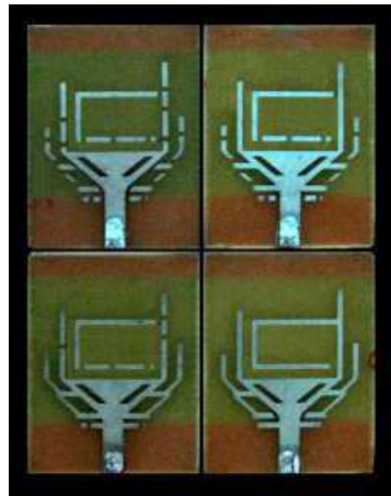
Figure 6. Fabricated prototype of proposed multifunctional antenna.
