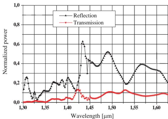
**Figure 3.** Normalized transmission and reflection spectra at the output port for the not optimized double bend.
