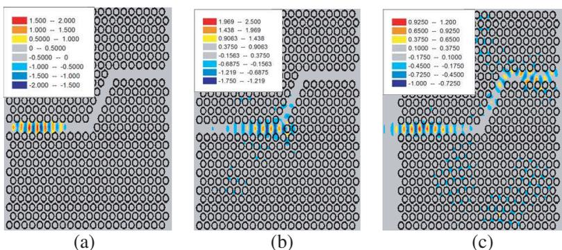
**Figure 4.** The distribution shape of the magnetic field Hz excited in TE mode. (a) For 15000 iterations. (b) For 20000 iterations. (c) For 30000 iterations.
