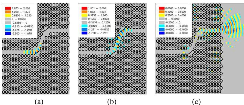
**Figure 7.** The distribution shape of the magnetic field  $H_z$  of the optimized bends excited in TE mode. (a) For 15000 iterations. (b) For 20000 iterations. (c) For 30000 iterations.
