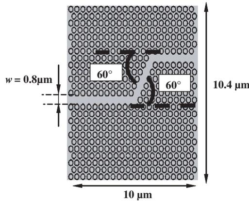
**Figure 2.** Layout for the FDTD modeling of the transmission through a double bends PhC waveguide. The photonic crystal is a triangular lattice of air holes ( $r = 0.348a$ ) in a dielectric medium ( $\epsilon = 10.5$ ). The W1KA PhC waveguide is obtained by removing 1 row of air holes.
