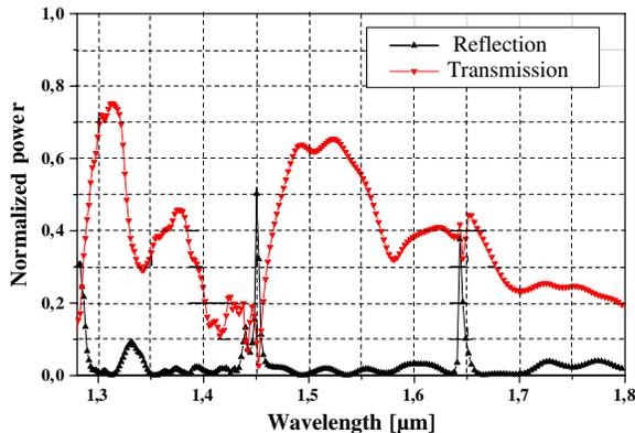
**Figure 6.** Spectral response in transmission and reflection of the optimized double bends obtained by the two-dimensional finite difference time domain (FDTD) simulation.
