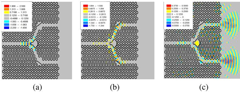
**Figure 10.** The distribution shape of the magnetic field  $H_z$  of the optimized splitter excited in TE mode. (a) For 15000 iterations. (b) For 20000 iterations. (c) For 30000 iterations.
