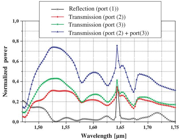
**Figure 9.** Computed transmission and reflection spectra of the optimized splitter obtained by the two-dimensional finite difference time domain (FDTD) simulation for the structure illustrated in Fig. 8. The electromagnetic power in the output port splits almost equally into the two PCW output ports throughout the waveguiding band.
