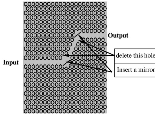
**Figure 5.** Topology optimization design of the double bend.
