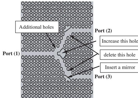
**Figure 8.** Topology optimization design of the splitter.
