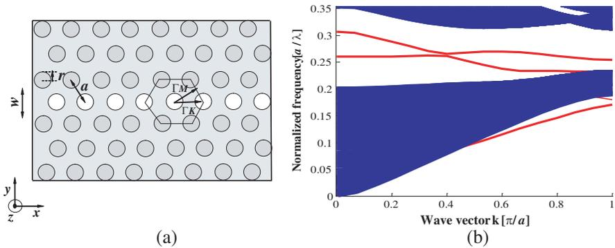
**Figure 1.** (a) Design of the triangular photonic-crystal waveguide. (b) Dispersion curves of the guided modes in a W1KA PhC waveguide.
