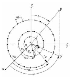
Figure 1. Concentric ring array antenna in X-Y plane.
