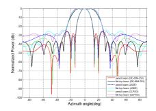
Figure 4. Normalized power patterns in dB for pencil beam+flattop beam configuration.
