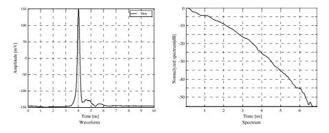
Figure 3. Pulse generator output waveform and spectrum.
