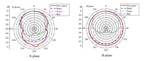
Figure 7. Normalized peak to peak voltage in dB vs. azimuth in degrees.
