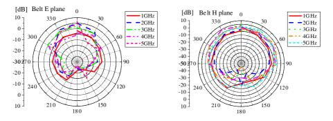
**Figure 9.** Radiation patterns at selected frequencies, belt scenario, E and H planes.
