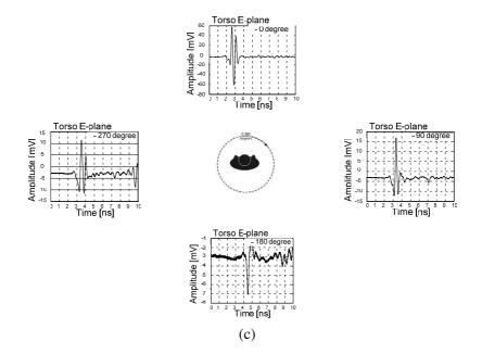
Figure 6. Example of measured time signals at 0, 90, 180 and 270 degrees for three scenarios (*E*-plane), (a) head, (b) torso, and (c) belt.
