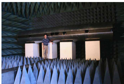
Figure 2. Slotted cylinder in anechoic chamber (floor covered, no ground plane).
