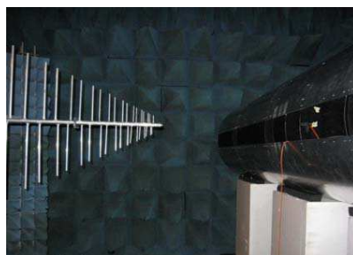
Figure 3. Slotted cylinder in anechoic chamber relative to LPDA.
