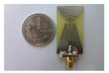
Figure 3. Photograph of the proposed antenna 2.
