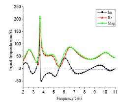
Figure 7. Input impedance of antenna 2.
