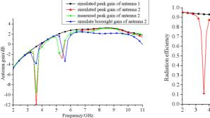
Figure 11. Antenna gain of the proposed antenna.
