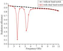
Figure 12. Simulated radiation efficiency of the proposed antenna.
