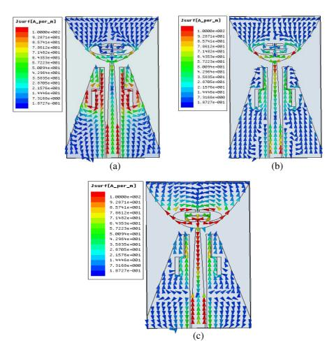
**Figure 6.** Simulated surface current distributions for antenna 2 at (a) 3.5 GHz, (b) 4.5 GH, (c) 5.5 GHz.
