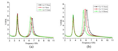
**Figure 9.** Simulated VSWR for antenna 2 with (a) different ra and (b) different Lr.
