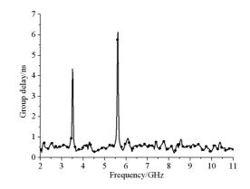
Figure 13. Measured group delay of the proposed antenna.
